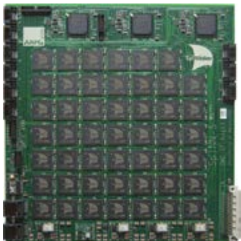
Figure 2: A SpiNNaker circuit board incorporating 48 chips, totalling 864 ARM processors.
